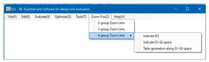
[Zoom Pos] Menu function searches zoom lens movement to yield the indicated EFL for infinite conjugate of mechanically compensated zoom lens.
